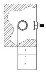
X: FLOW/CLIP: Min. 44 mm. / Max. 64 mm.
