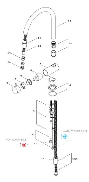
\* THE OPERATING AREA OF THE COUNTER-WEIGHT SHOULD BE FREE AND CLEAR FOR ITS CORRECT FUNCTIONING
